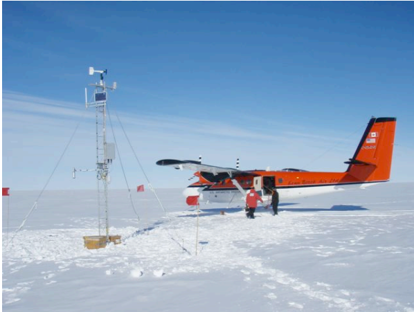
Figure 1. Margaret AWS site, as seen here during its installation in November of 2008, is scheduled for servicing in the coming field season.
