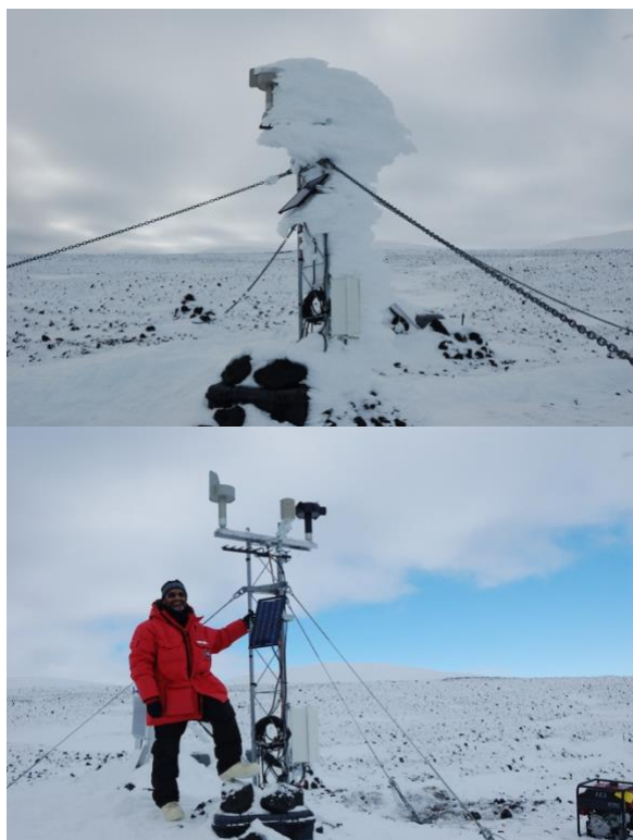
Figure 2. Before (top) and after (bottom) photos of Minna Bluff AWS taken during its servicing in early 2018. This is the second time icing this season on the AWS tower impeding its operation.
