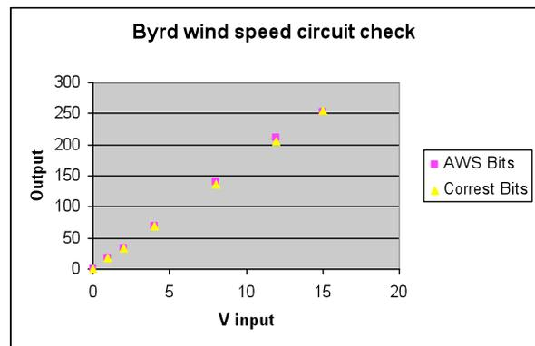
The overall accuracy of the wind speed circuit was within 2% after 30 years.
