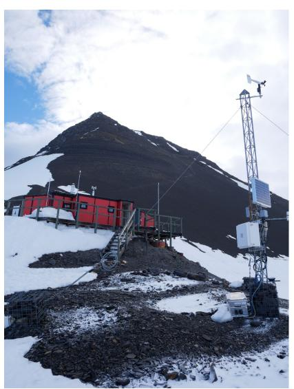
SR50 sonic ranger transducer head replaced.
