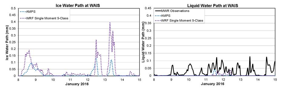
AMPS and PWRF 3.9.1 with WSM5C microphysics show much more ice water path than liquid water path.
